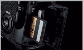
Images can be copied between SD cards within the camera, making image data backup possible without a PC.
