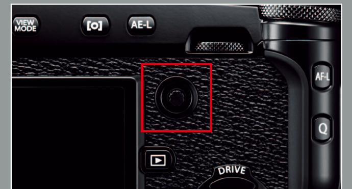
Clicking the focus lever in the centre will instantly return the focus area back to the central point.
