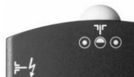
Measurement by the incident method is far more accurate and reliable to establish the correct exposure setting than the calculating of a mean value obtained with the reflected light measurement in your camera. In the latter case, the reading depends upon the range of contrasts of the subject.
